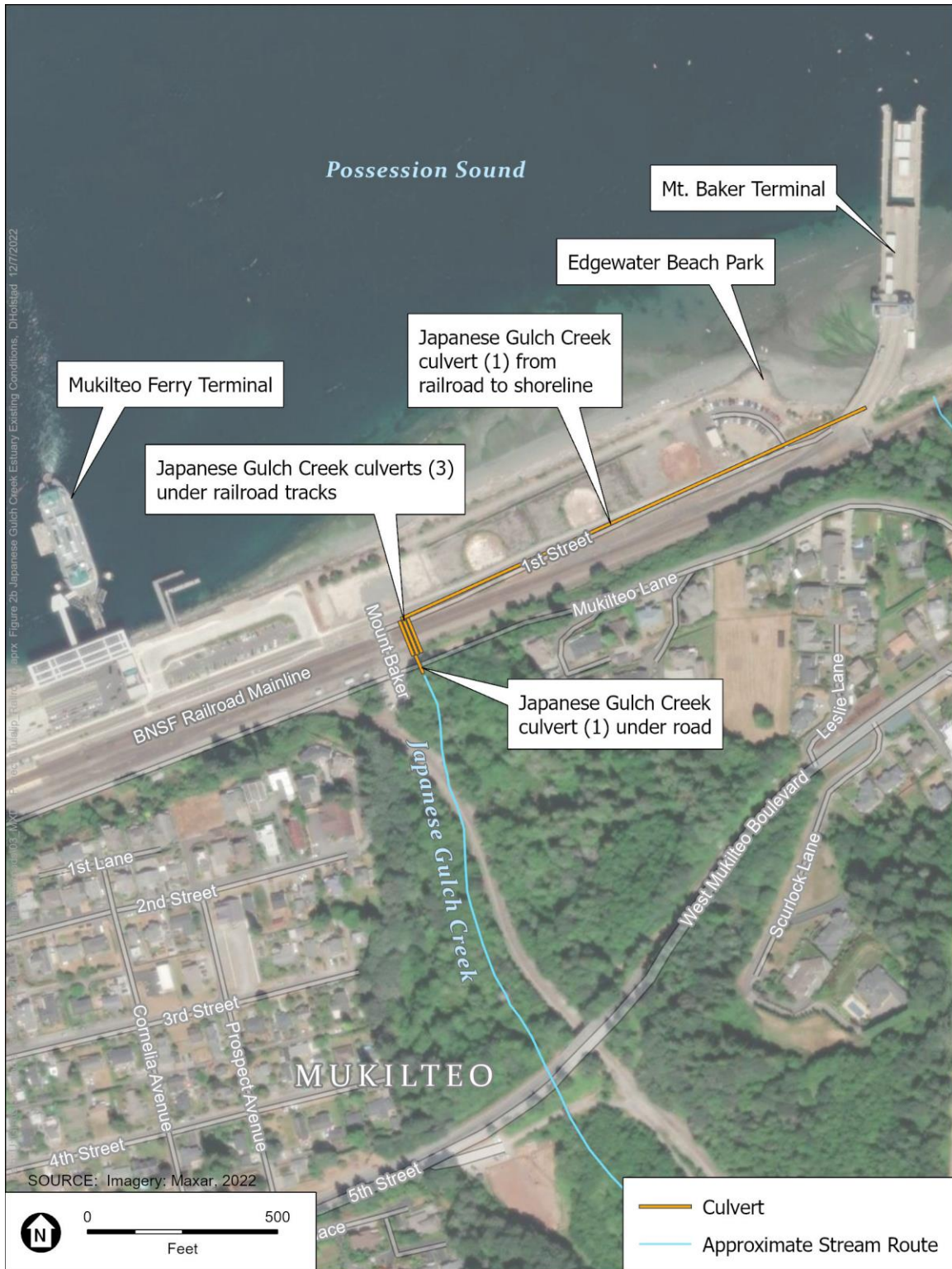
Figure 16. Japanese Gulch Creek Site Showing Culvert Network of Lowermost Creek Section
