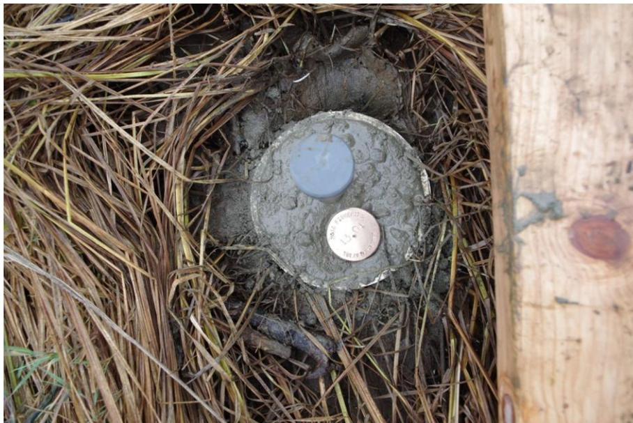
Figure 3.3. Capped SET mounting receiver and copper survey marker.
