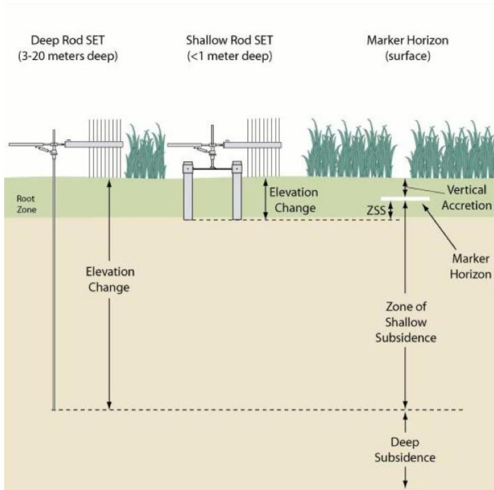
Figure 3.1. Rod surface elevation table - marker horizon (RSET-MH) in both shallow and deep configurations. All installations associated with the current work will be deep.
