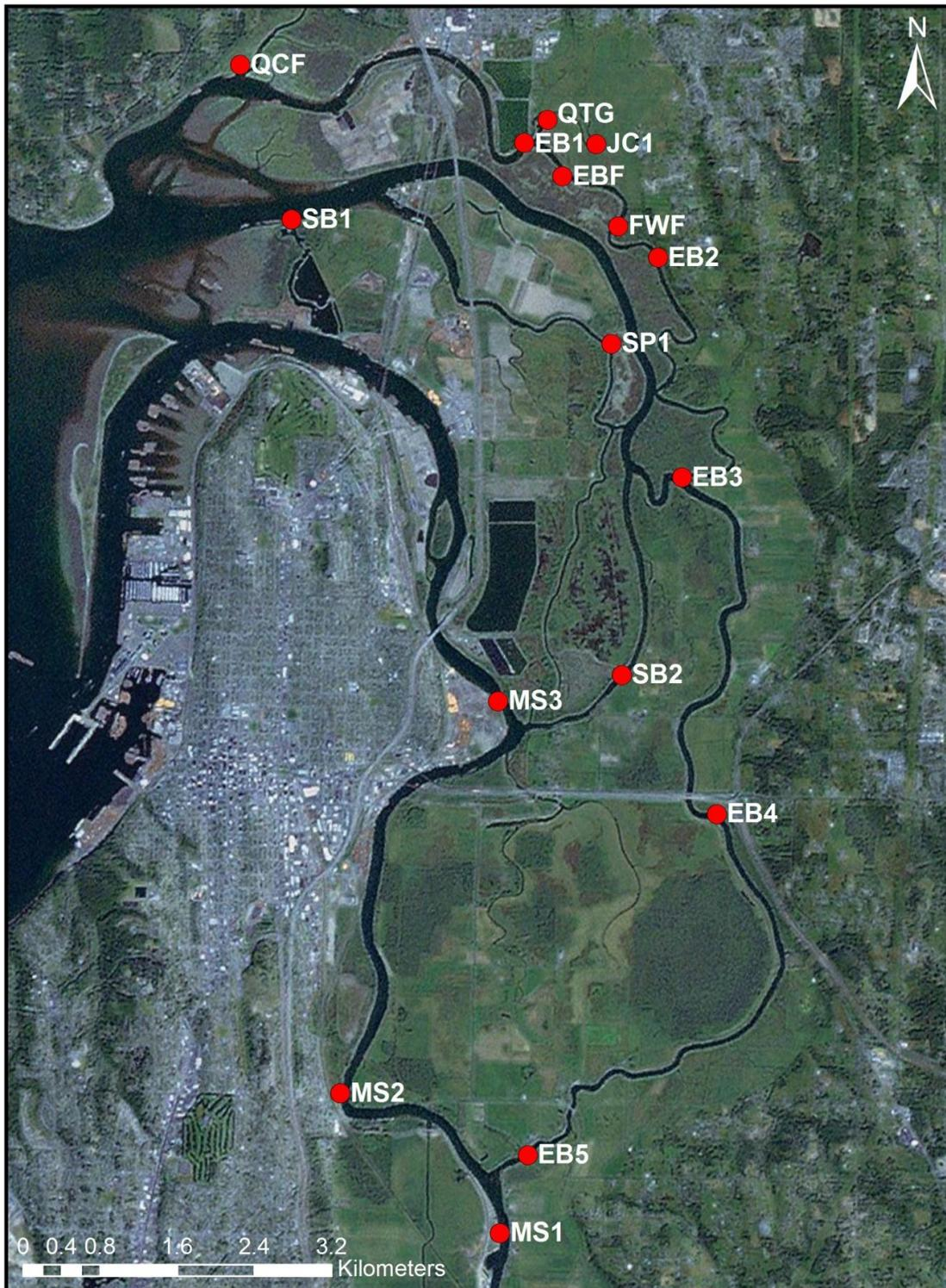
Figure 4.1: Locations of continuous (10-minute interval) water elevation, temperature, and salinity monitoring points within the Snohomish River estuary.
