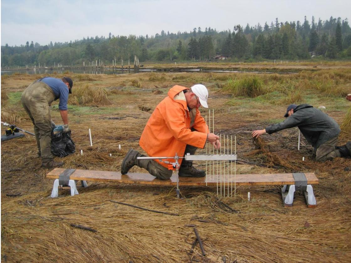
Figure 3.4. Measuring surface elevation with rods at one of four positions for each location. Fieldspare marker horizons being installed at the four corner locations of the SET plot indicated by four short PVC pipes.
