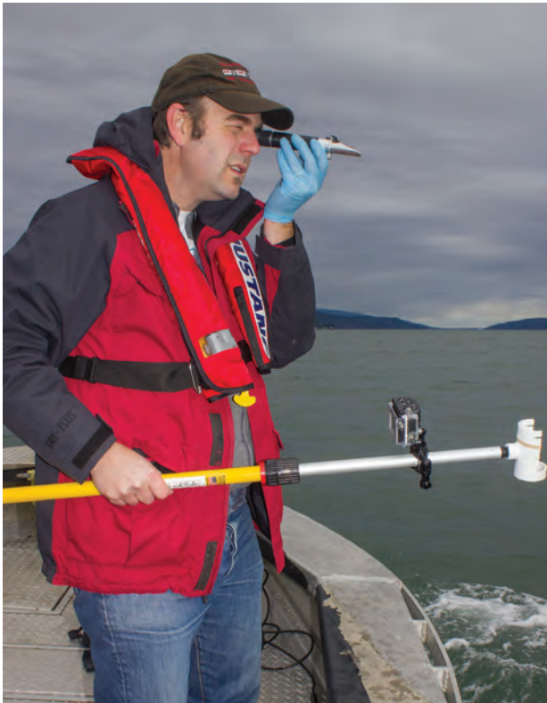
Seth Book, Skokomish Tribe water quality biologist, uses a refractometer to measure the salinity of a water sample from Hood Canal.
