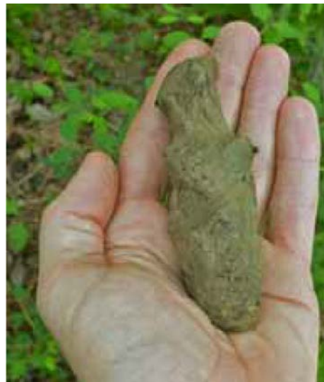
Soil Hand Texture Test : Sand vs. Clay (WSU Rain Garden Handbook)
